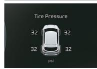
Displays real-time tyre pressure information and alerts if the pressure falls during uphill climb from standstill
